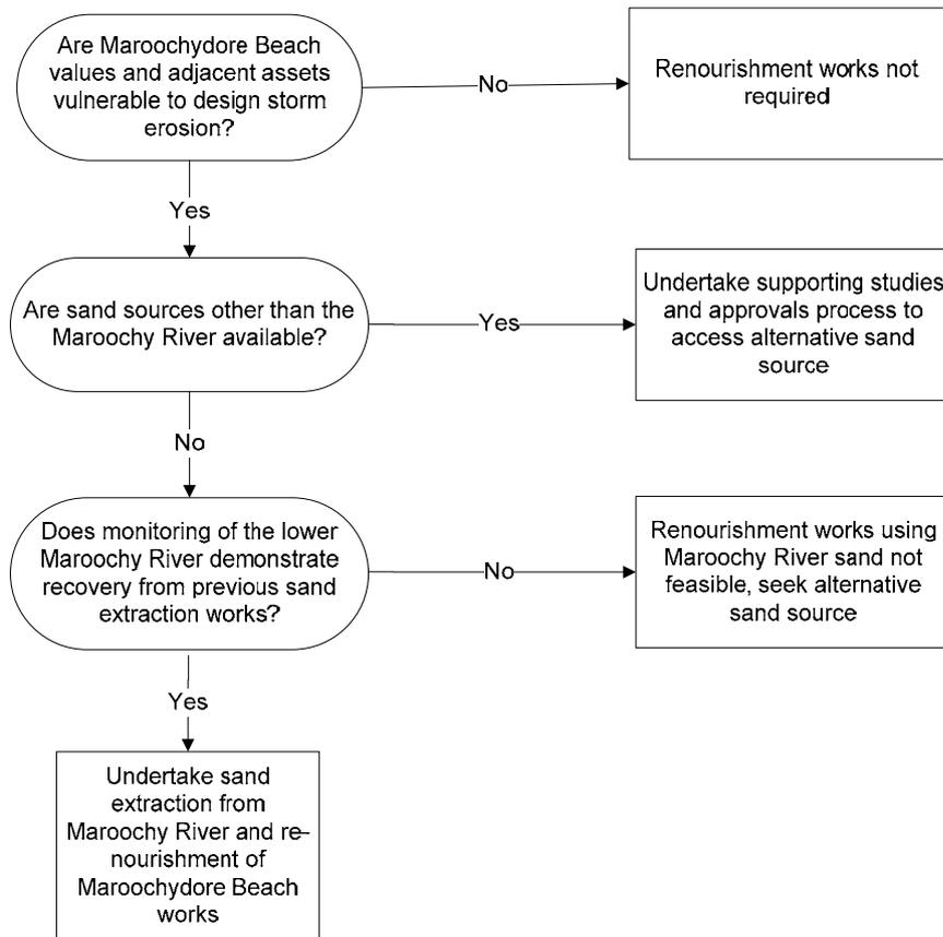
**Figure 4-1 Decision Tree for Determining the Need and Feasibility of Future Re-Nourishment Works**
