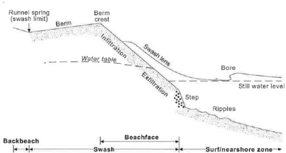
**Figure 2-3 Schematic Diagram of Swash Zone and Beachface Morphology
