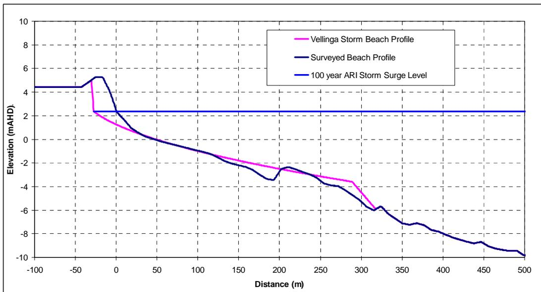
**Figure 2-2 Example of Predicted Storm Erosion Profile**
