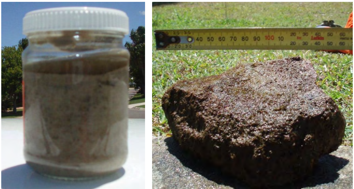
Figure 2-3 Sand with minor fines & Rock protection greater than 75mm .
