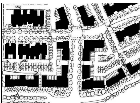
Figure SC6.3I Perimeter block form
