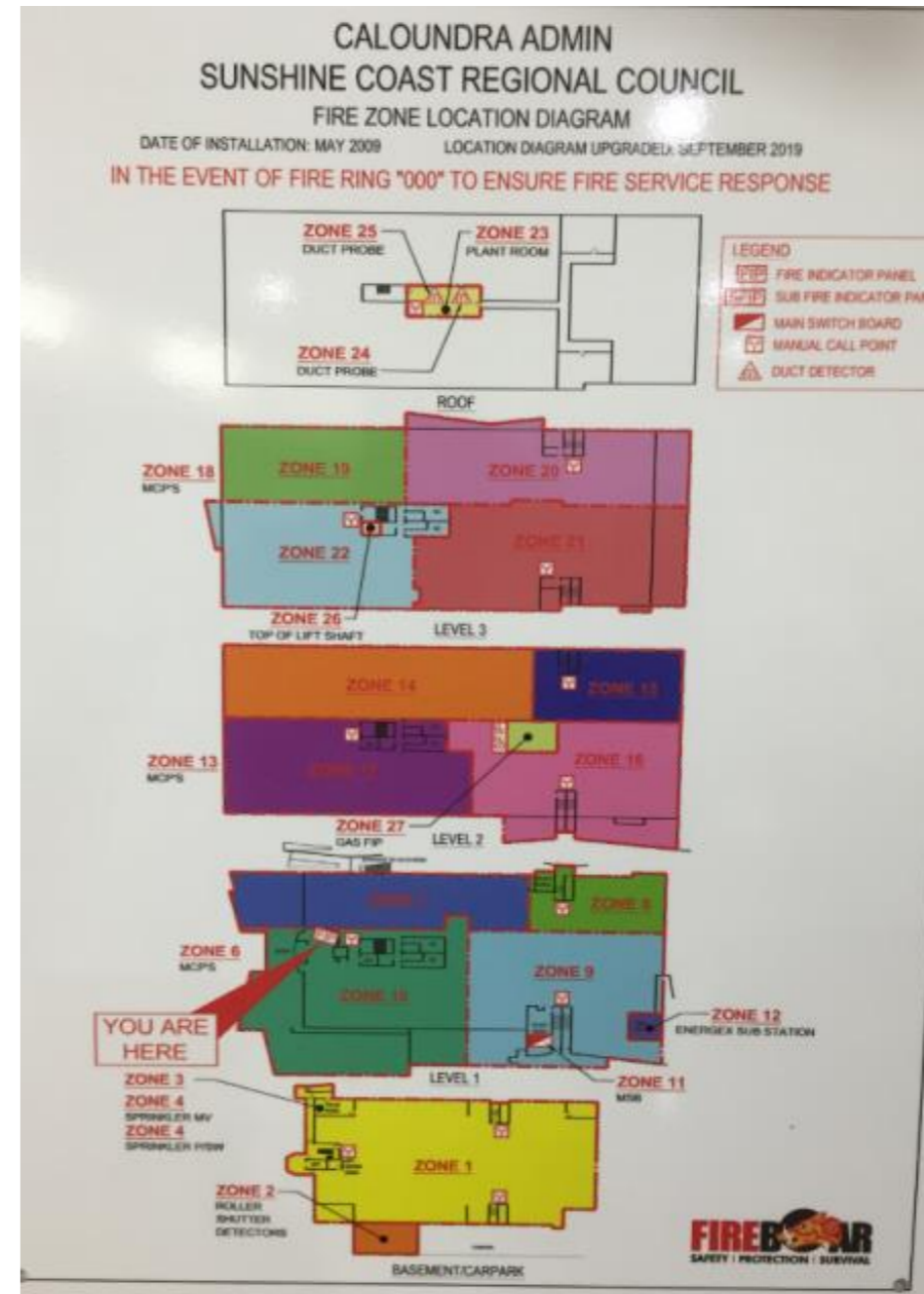
Figure 20 - Administration Building Detection Zone Location Diagram
