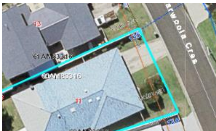
Carport located over Unitywater sewer (orange line)
