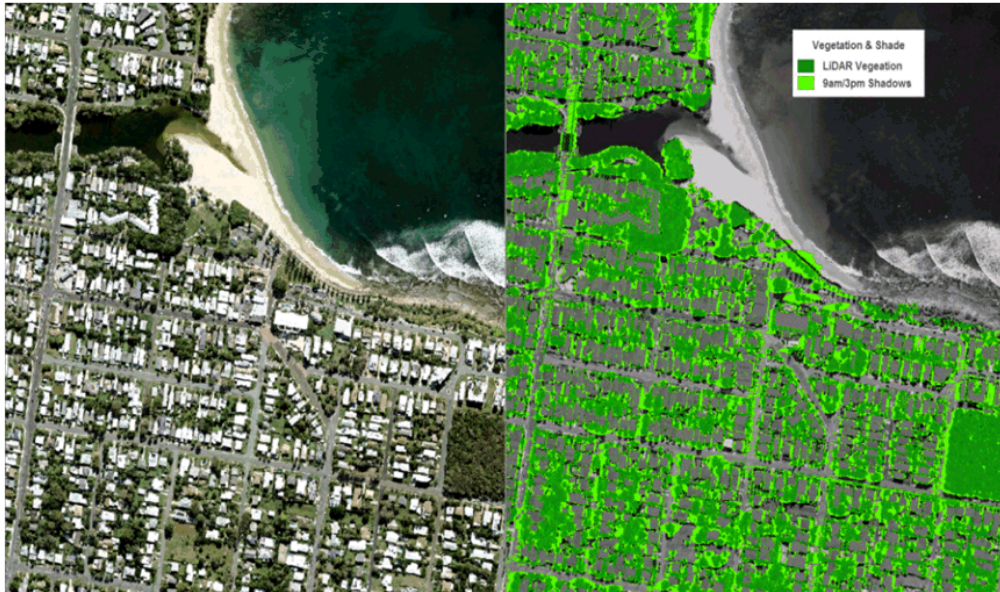
Figure 5: Shade is calculated using tree height and time of day within mapping software. The left image shows standard aerial photography, the right image, a LIDAR derived vegetation map with trees (non-ground vegetation) in dark green, and the 9am/3pm summer shadows in light green.
