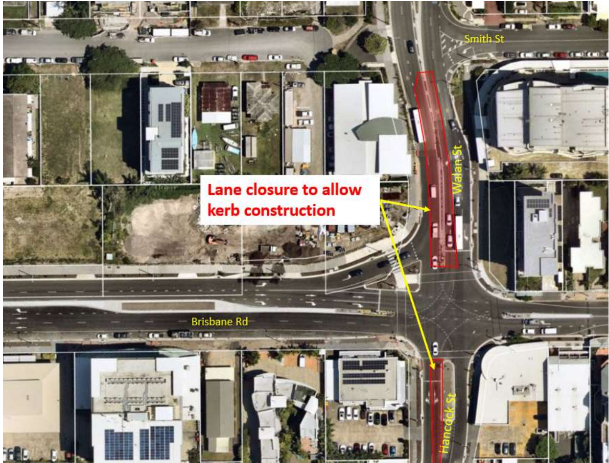
Figure 1. Walan Street - Concrete median construction area with partial lane closure. Hancock Street - Partial lane closure for traffic movement purposes only. Temporary changes to traffic conditions Monday to Friday only. All works are weather dependent.
