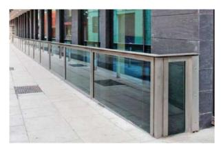
Figure 50 Glass flood protection panels – commercial application (<u>www.floodcontrolinternational.com</u>)
