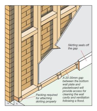
Figure 53 Recommend substituting plasterboard for fibre cement sheeting. Leave a gap at the base of fibre cement sheeting for drainage and ventilation. (H-N FMSC 2006a)
