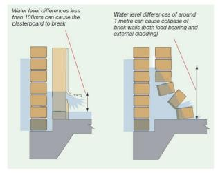
Figure 52 Internal plaster and cavity brick failure due to uneven water pressure (H-N FMSC 2006a)
