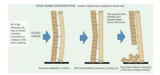
Figure 38 Typical brick veneer wall failure from flood forces (Hawkesbury-Nepean Floodplain Management Steering Committee, 2006)
