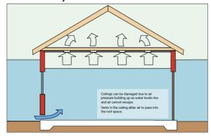
Figure 54 Use ceiling vents to reduce air pressure in a wet flood proofed building
