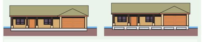
Raising the slab 500-800mm on waffle pods (right) is very effective in reducing the possibility of the house being innundated in situations of overland flooding and where there is greater risk of the drainage infrastructure being overwhlemed by intensive localised flooding and blockages.
