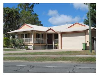
Figure 13 House with suspended timber flooring above defined flood level
