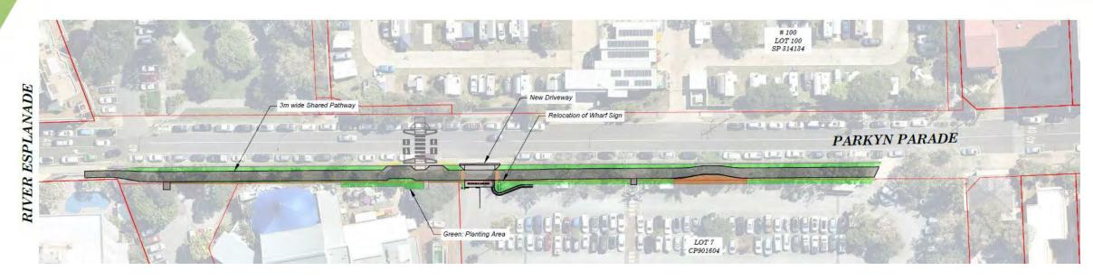
Parkyn Parade footpath renewal is being widened from 1.8m to 3m to meet the growing needs of off-street cyclists and pedestrians. The new shared pathway will be offset from the back of kerb by 1.2m to provide buffer between parked cars and pathway users.
