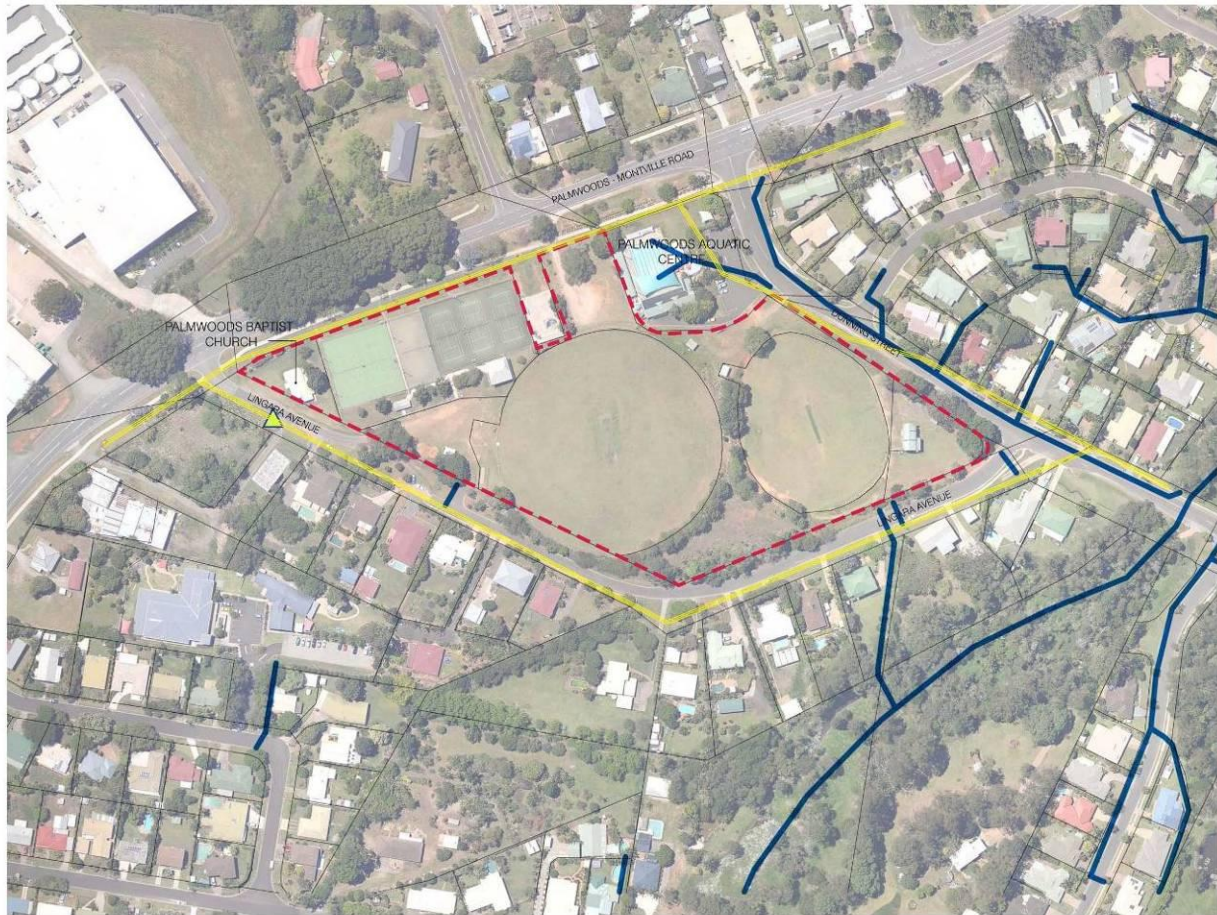
FIGURE 12 - STORMWATER INFRASTRUCTURE MAP
