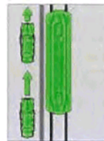
Tramway with separation kerb
