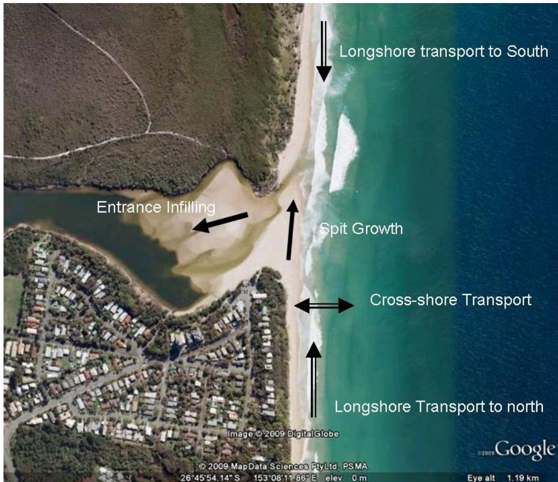
Figure 53: Lake Currimundi Entrance (June 2008) showing the dominant sand transport mechanisms
