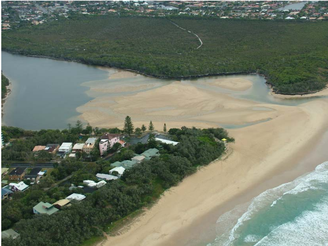
Figure 55: Entrance Channel forced to the north following the artificial build-up of the berm in August 2006
