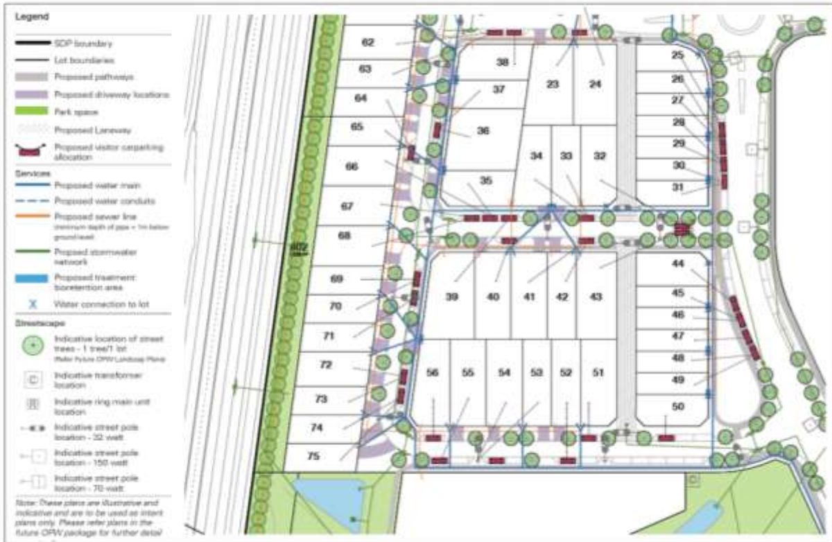
Figure 24: Consolidated infrastructure plan (refer to Maps 7A – 7I of Attachment B for larger images)
