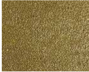
Integrally Coloured Concrete with Lightly Exposed Aggregate
