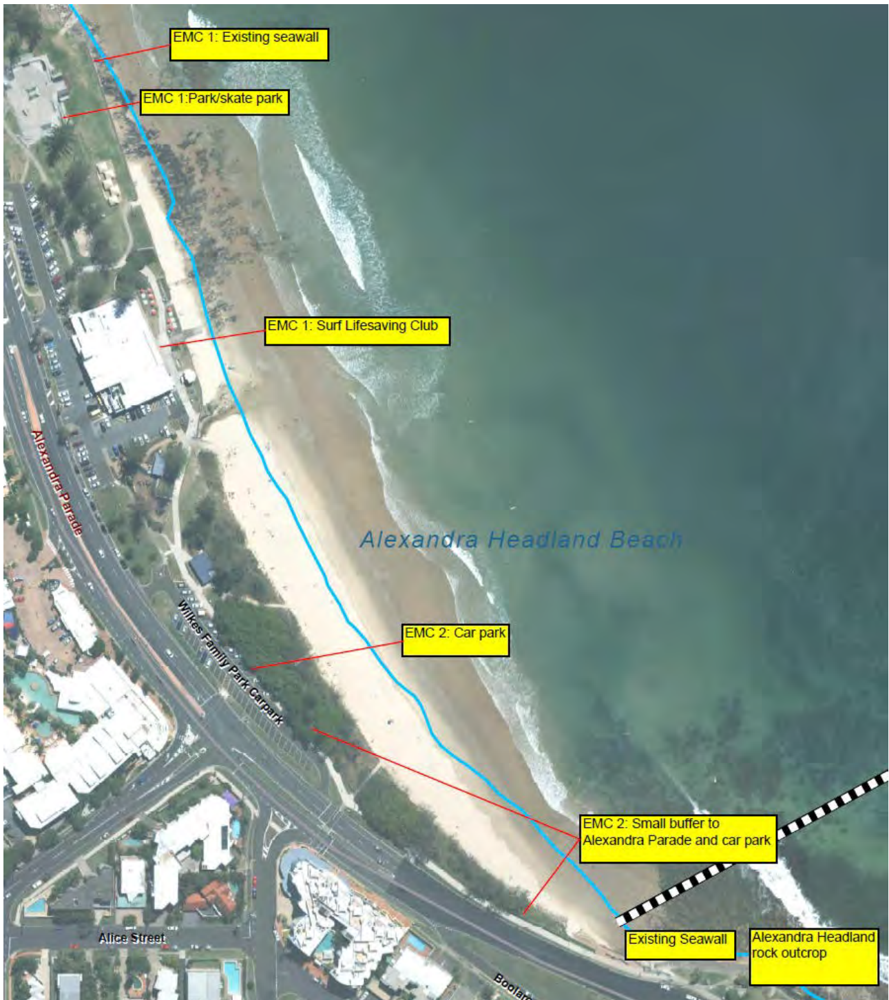
Figure 6.11: Annotated air photo showing the erosion management considerations for Alexandra Headland Beach
