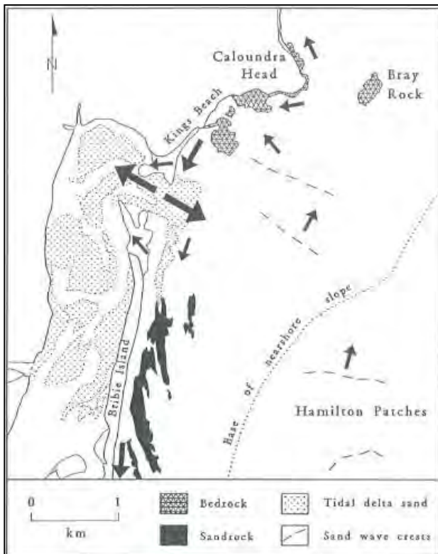
Figure 6.23: Sediment transport divide – sand transport to the north and south of Caloundra Head (from Jones 1992)
