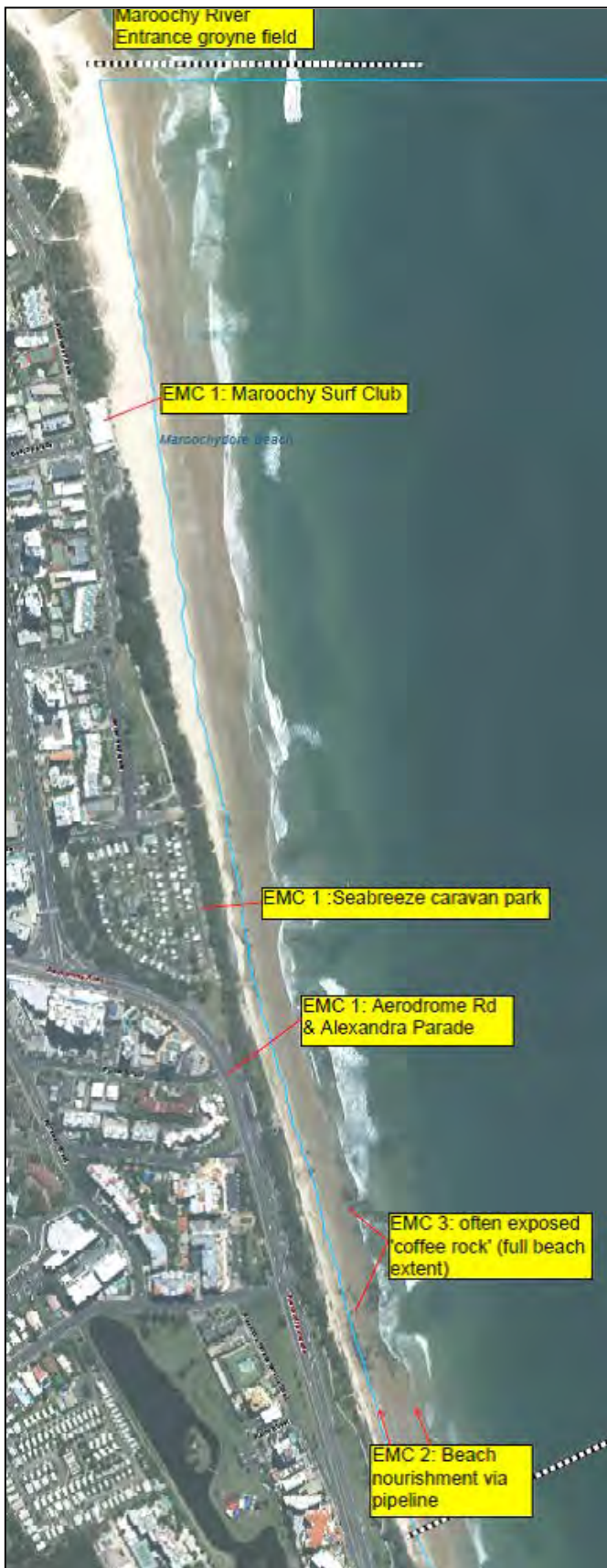
Figure 6.9: Annotated air photo locating the erosion management considerations for the Maroochydyore Beach Unit
