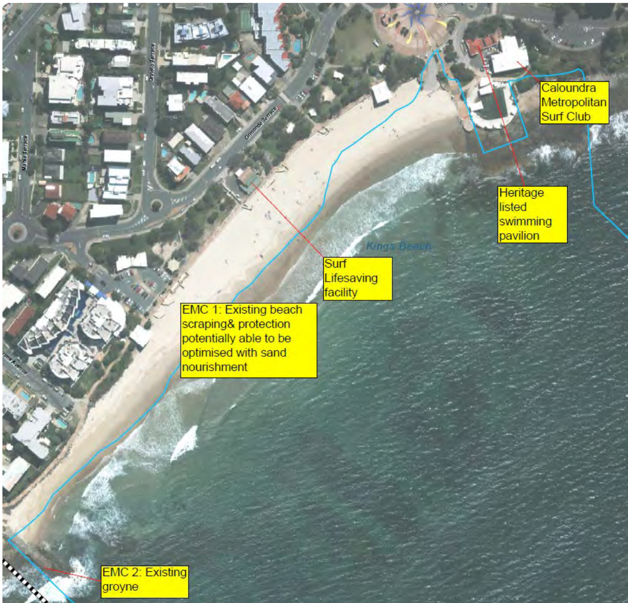
Figure 6.25: Annotated aerial image of Kings Beach showing listed erosion management considerations
