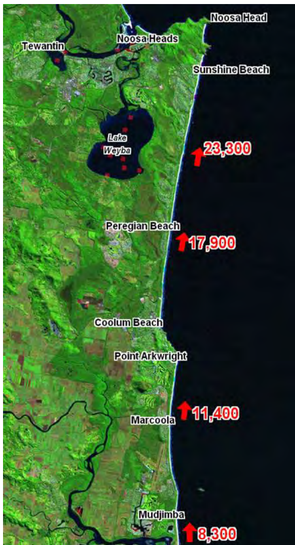
Figure 6.1: Potential net longshore sand transport rates (m 3 /yr) for Zone 1 and further north.
