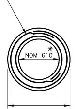
Overall diameter nom 1050\* Concrete thickness 35 or 50
