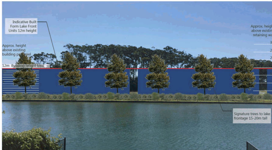
Figure 9: Code assessable development option showing 3 storey unit blocks with existing trees remaining.
