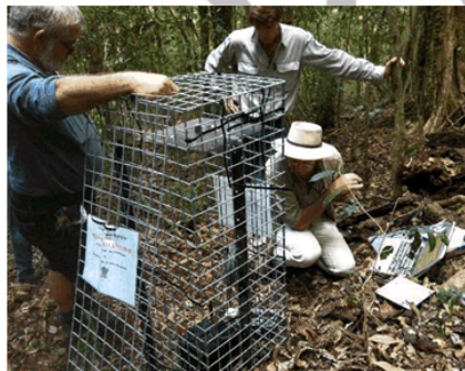
Solar powered acoustic survey equipment installed on an environmental reserve to detect endangered birds. Equipment developed by local engineers in partnership with leading acoustic software experts from a university in Japan.
