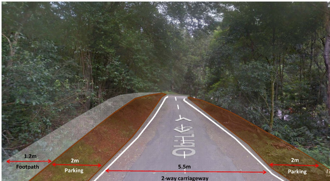
Figure 4. Option 3. Two way carriageway allows safe movement for vehicles. Parking to both sides of lane. New pedestrian path. Would potentially require land acquisition and tree removal and replacement.
