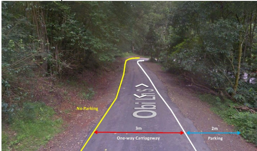
Figure 2. Option 1. One way carriageway with parking limited to 1 side. Passing vehicles must utilize the no parking side.
