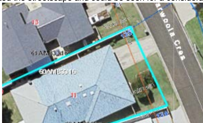
Carport located over Unitywater sewer (orange line)
