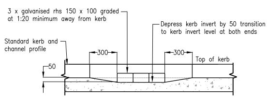
TREE PIT KERB INLET ELEVATION
