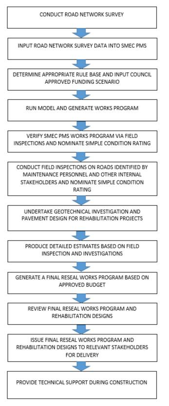
Figure 24: Flow chart to generate reseal works program
