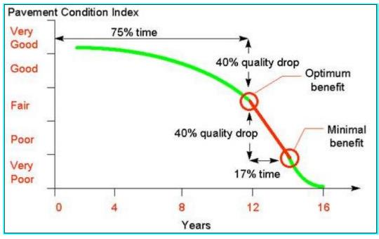
Figure 25: Typical form of asset deterioration curve
