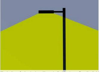
Illustration of a luminaire with controlled luminous flux; the light is emitted below the horizontal plane, reducing sky glow
