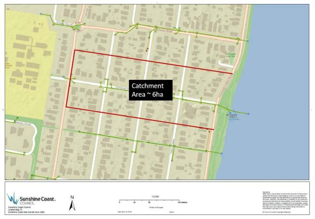
Figure 4 – Catchment area treated by Earnshaw Street Vegetated Infiltration Basin
