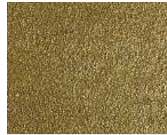
Integrally Coloured Concrete with Lightly Exposed Aggregate
