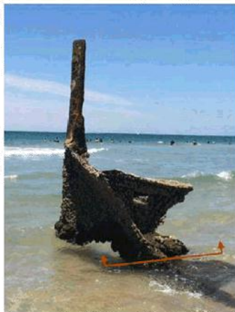
Figure 44. Indicative cut for the removal of the stern assembly. View from the starboard side. (Cosmos Archaeology, 19 December, 2014)
