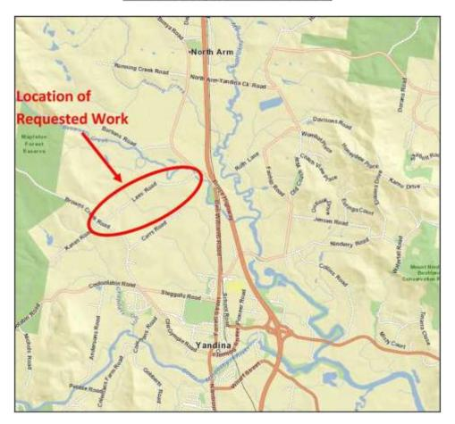
Lees road is currently sealed for the first 0.2kms from the east and the first 50m from the west, the remaining 1.7kms in the middle is unsealed. The proposal is for the sealing of the remaining 1.7kms, creating a continuous bitumen sealed pavement connecting Browns Creek Road to the west and Bunya Road to the east.
