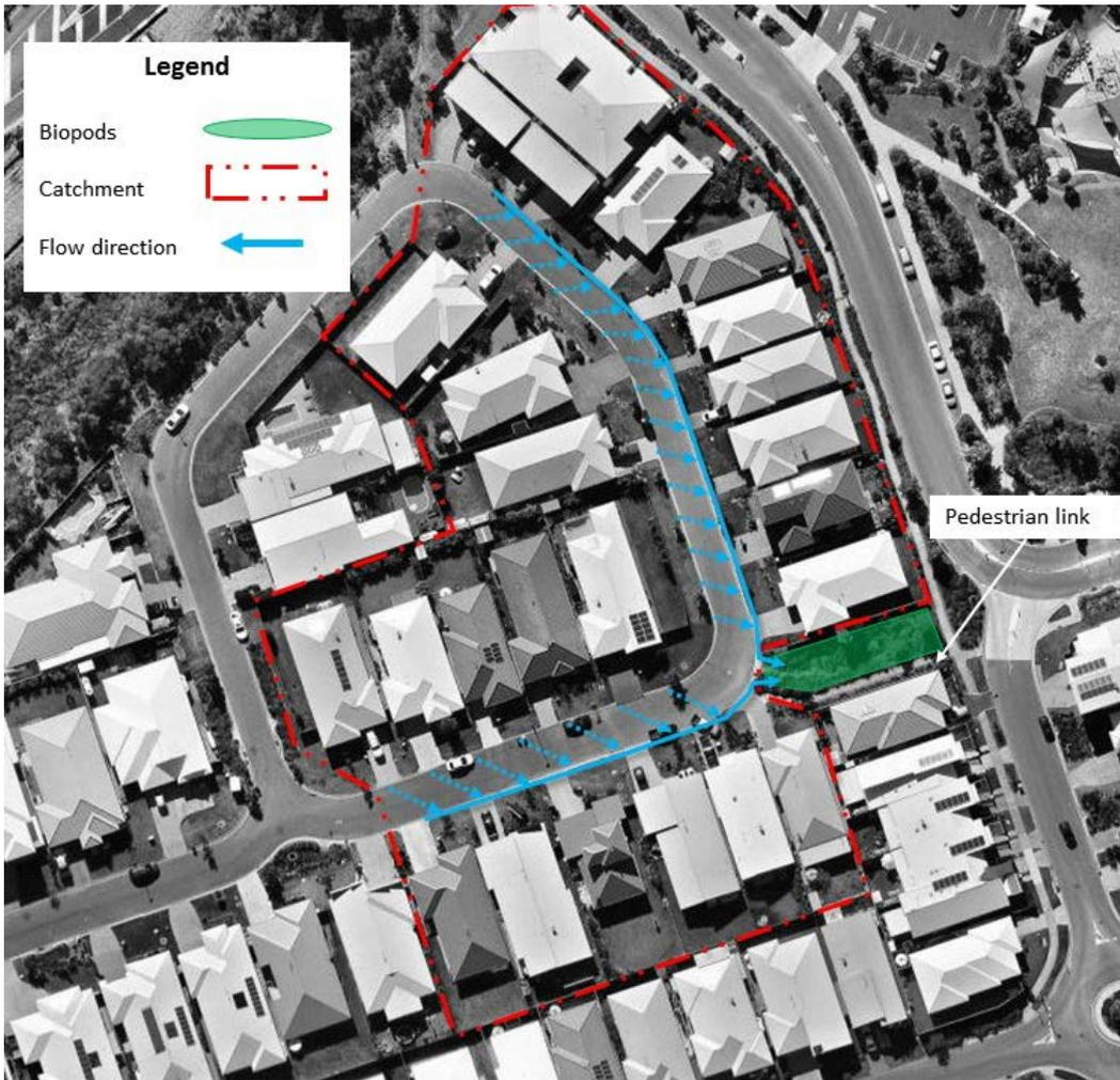
Figure 8 Biopod Located with Pedestrian Link (1-Way Crossfall)
