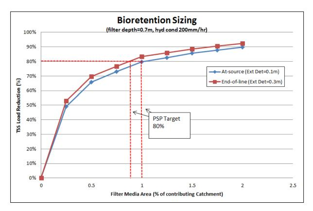
Figure 3.1 – Bioretention Performance Curves
