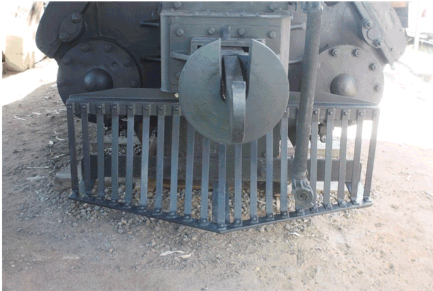
Replica cowcatcher similar to that fitted when the Buderim Tramway Krauss locomotive was built in 1914. 19 July 2016. Image: D J Mewes
