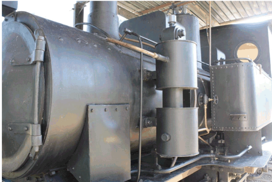
Mock-up of a Westinghouse Pump as fitted to the Buderim Tramway Krauss locomotive at Wise's Farm, Maroochydore. 19 July 2016 Image: D J Mewes
