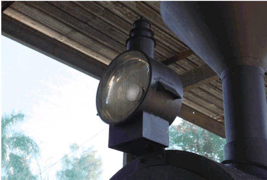
Replica headlight on the Buderim Tramway Krauss locomotive. 19 July 2016. Image: D J Mewes
