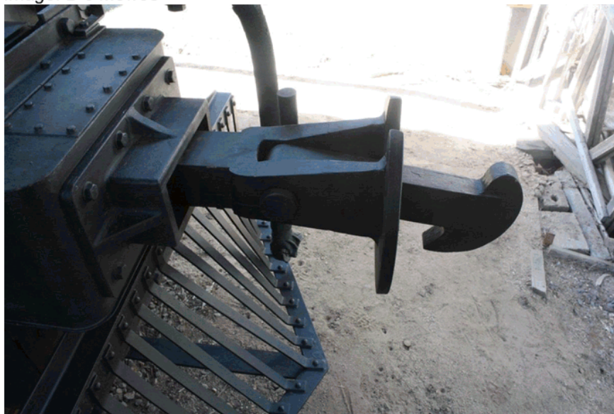
Replica "chopper" coupling made from timber as fitted to the Buderim Tramway Krauss locomotive. 19 July 2016 Image: D J Mewes
