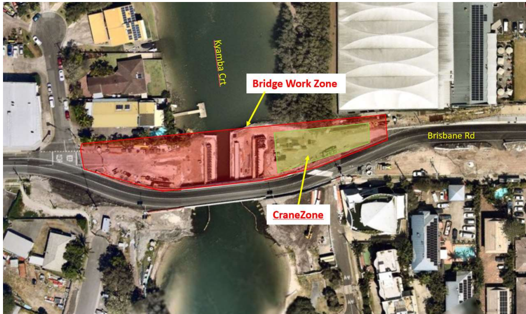
Figure 1. Location of Mayes Canal Bridge under construction – Brisbane Road Temporarily reduced clearance for marine vessels.
