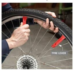
Once one side of the tyre is off, remove inner tube and tyre from rim - remove inner tube from tyre. Position tyre for easy reference to potential puncture site.
