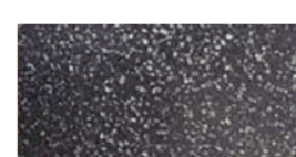
CCS Liquorice (8.3% oxide rate) with (Boral) 'Salt and pepper' aggregate (70% white and 30% black)
