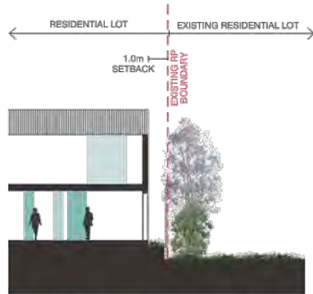
SECTION A - RESIDENTIAL ADJACENT TO EXISTING RESIDENTIAL
