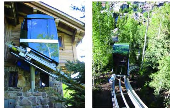
Example of mini-funicular system installed to a private residence in Vail/USA
