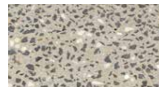
Plain concrete with (Boral) 'Salt and pepper' aggregate
