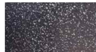
CCS Liquorice (8.3% oxide rate) with (Boral) 'Salt and pepper' aggregate (70% white and 30% black)
