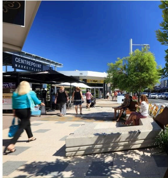
P 06 The materials are inspired by the colours and textures of Caloundra. Footpaths feature exposed aggregate concrete with muted earthy tones and textures. Timber-clad bespoke seating and interpretative elements are used along the street to mark places to rest and watch.
