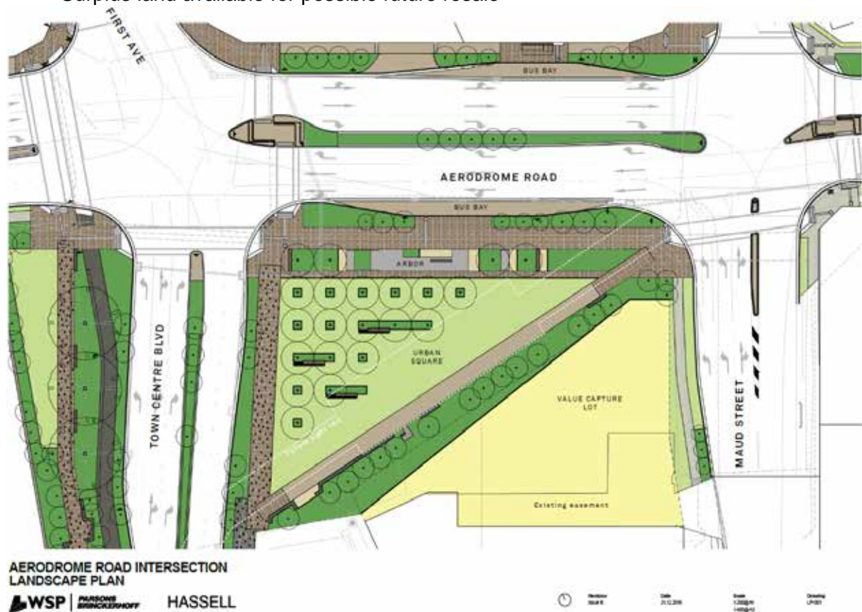
FIGURE 2 – Intersection Upgrade General Arrangement
