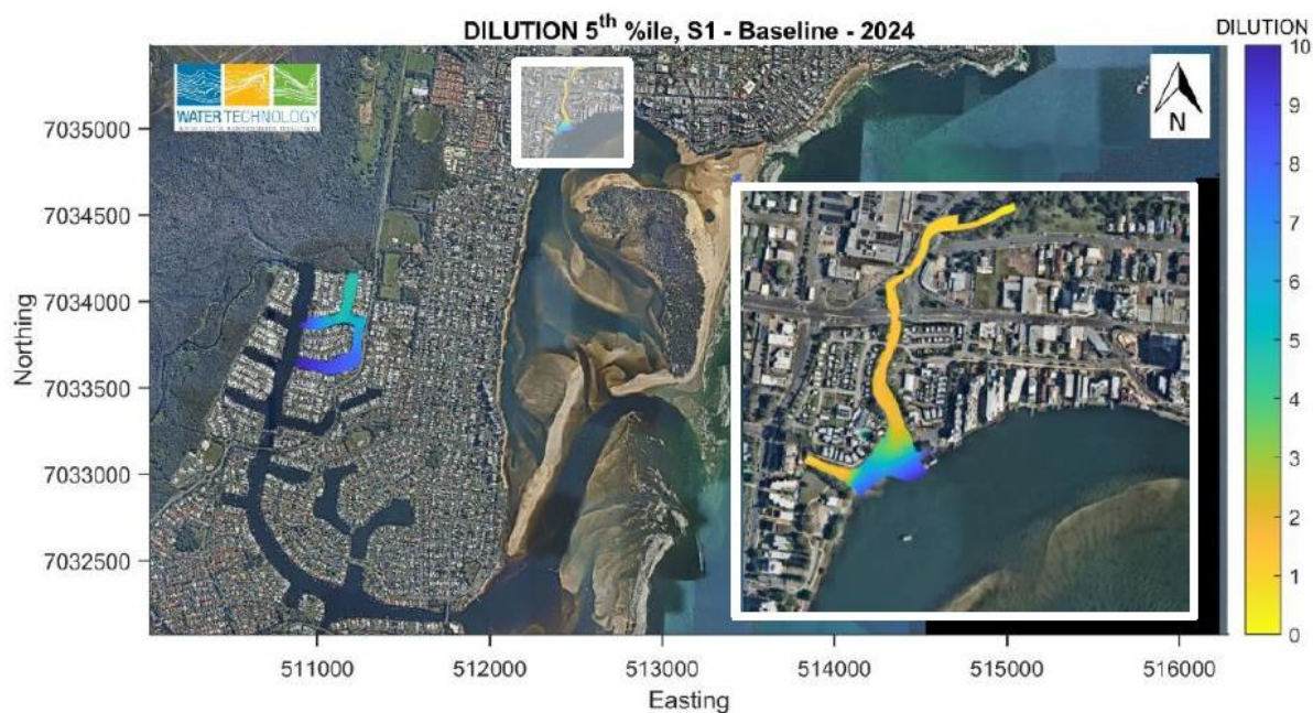
Figure 20 5 th Percentile 1:10 dilution extent for baseline (pre-construction) scenario 2024
