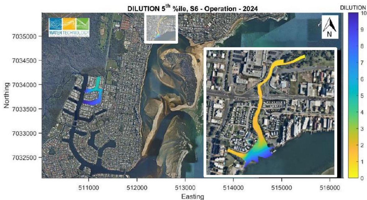
Figure 21 5 th Percentile 1:10 dilution extent for operational scenario 2024
