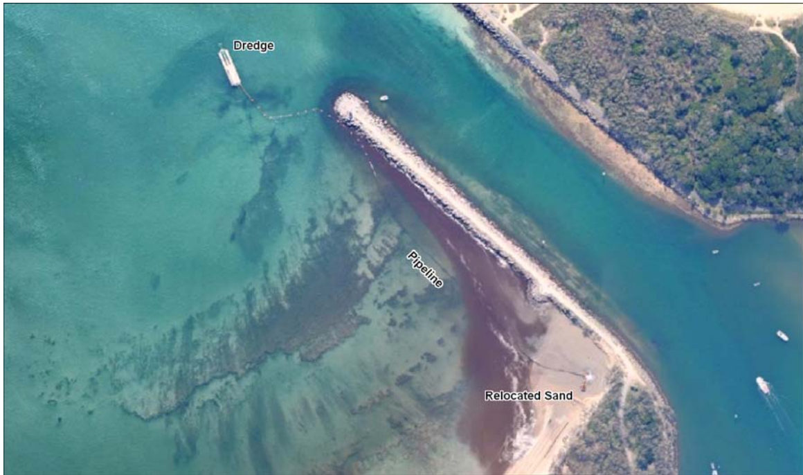
Figure 3-2 Dredger Relocating Sand from the Mooloolah River Entrance to Mooloolaba Beach via a Pipeline (Source: NearMap, 2011)
