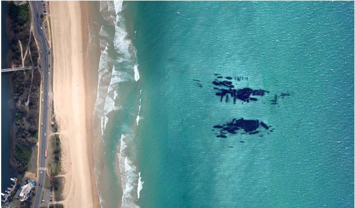
Figure 3-7 Geotextile Sand Container Artificial Reef at Narrowneck, Gold Coast (Source: NearMap, 2011)
