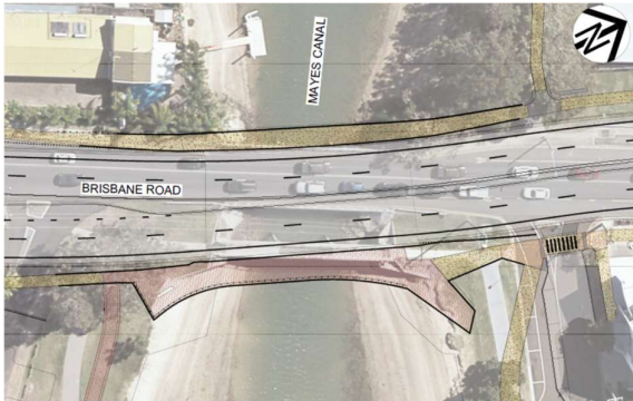
Figure 4 Footprint of new Mayes Canal Bridge. Old bridge to be demolished after new bridge constructed.
