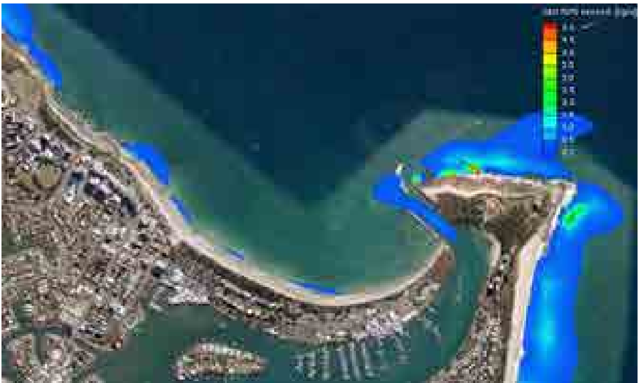
Figure 3-45 Spring Tide Period Median Sediment Transport with Wave Case 1: H_s = 3m , T_p = 12s , Dir = SE
