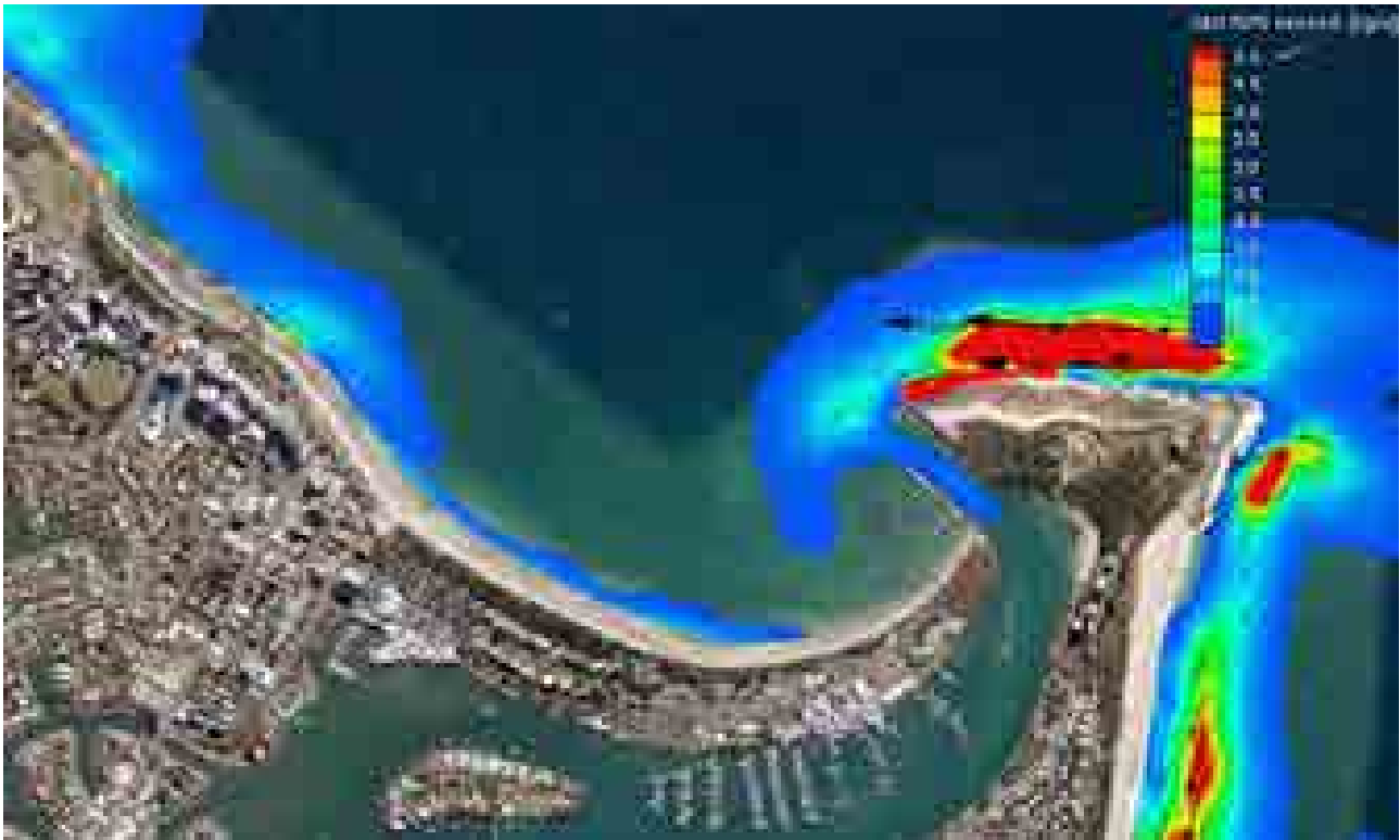
Figure 3-46 Spring Tide Period Median Sediment Transport with Wave Case 2: H_s = 3\text{m} , T_p = 12\text{s} , Dir = E
