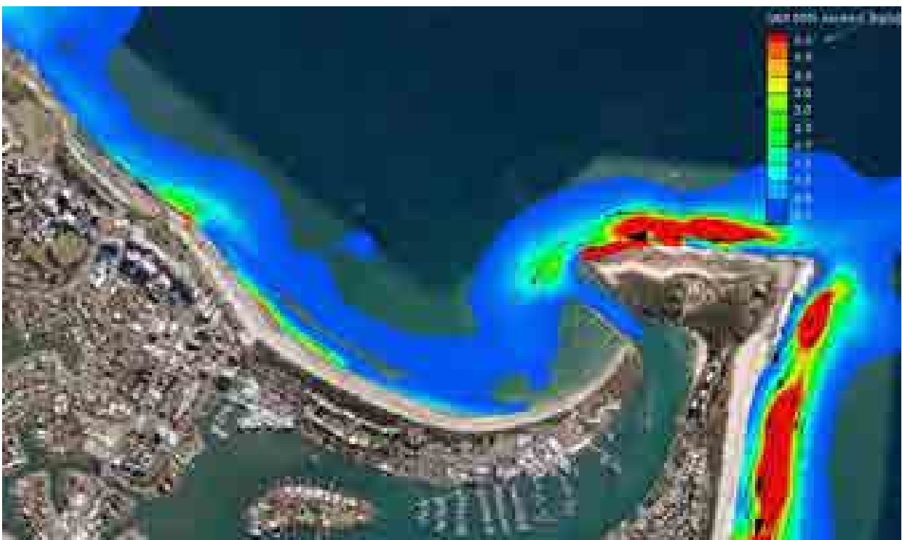
Figure 3-47 Spring Tide Period Median Sediment Transport with Wave Case 3: H_s = 3\text{m} , T_p = 12\text{s} , Dir = NE
