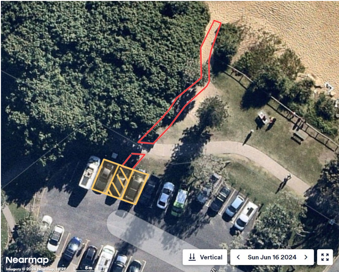
Proposed layout (coloured concrete ramp in red and new DDA carparks in yellow with blank out space for compliance)
