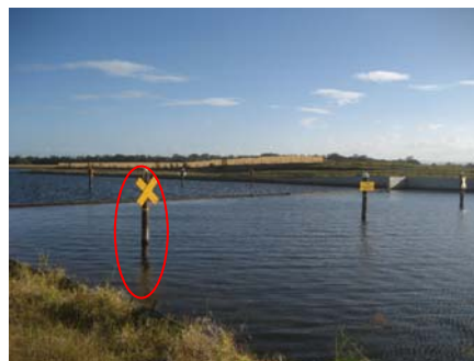
Figure A9.38: Tide gauge No.4 (TWR-2050 Serial: 12537) in the Lake Kawana near the weir
