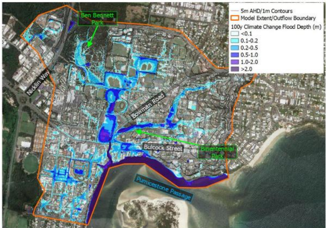
Figure 4.4 Existing 1% AEP floodplain extent
