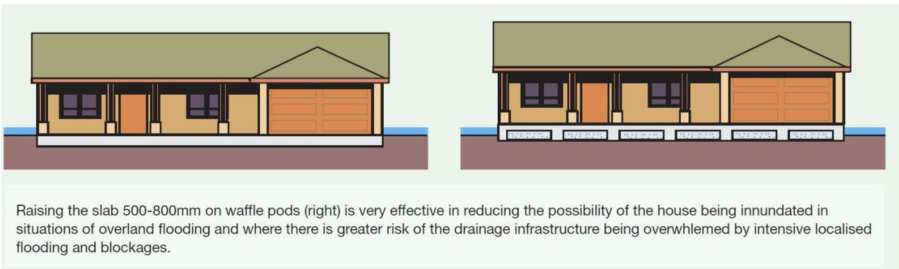
Figure 22 Elevated slab on ground illustration<sup>18</sup>
