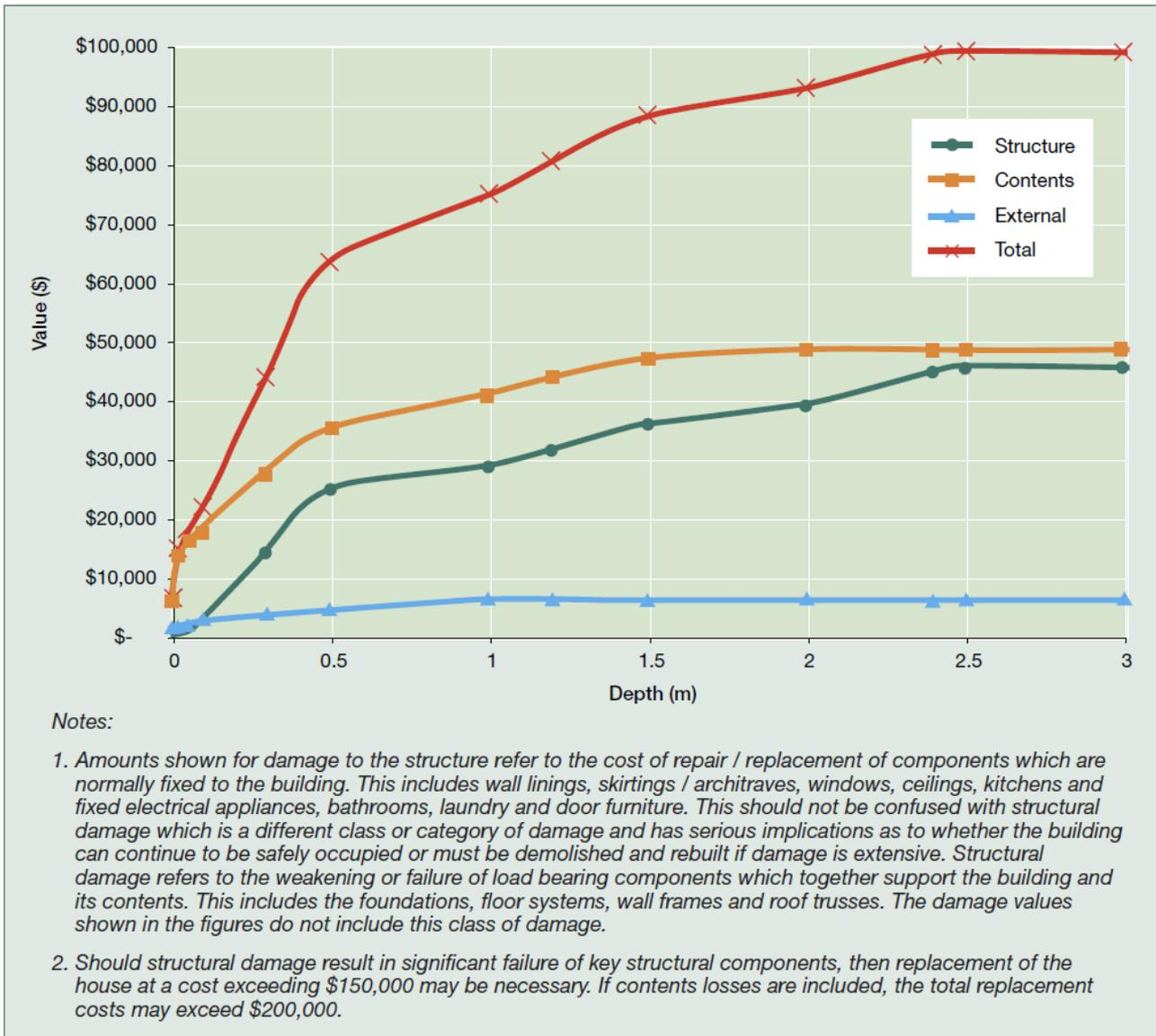
Figure 1 Damage in dollars for a single storey house verses depth of inundation in metres (Hawkesbury-Nepean Floodplain Management Steering Committee, 2006)
