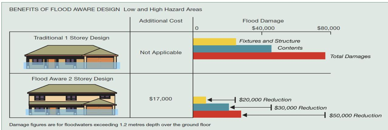
Figure 21 Reduction in overall food damage due to additional house storey<sup>17</sup>
