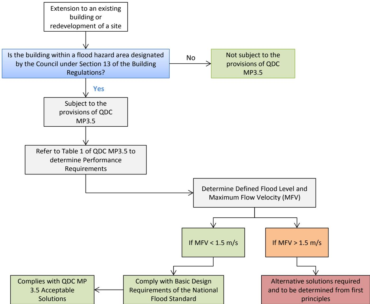
Figure 10 Process for determining the application of QDC MP 3.5
