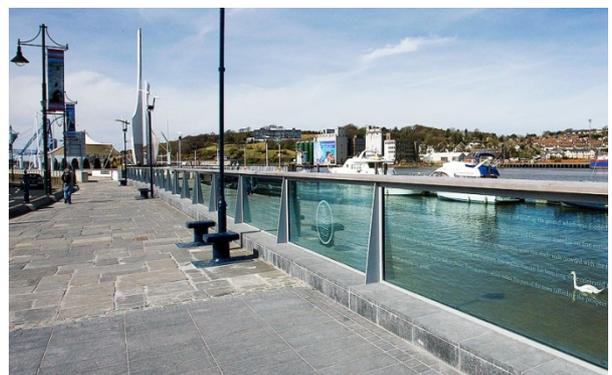
Figure 37 Glass flood protection panels ([www.careyglass.com](http://www.careyglass.com))
