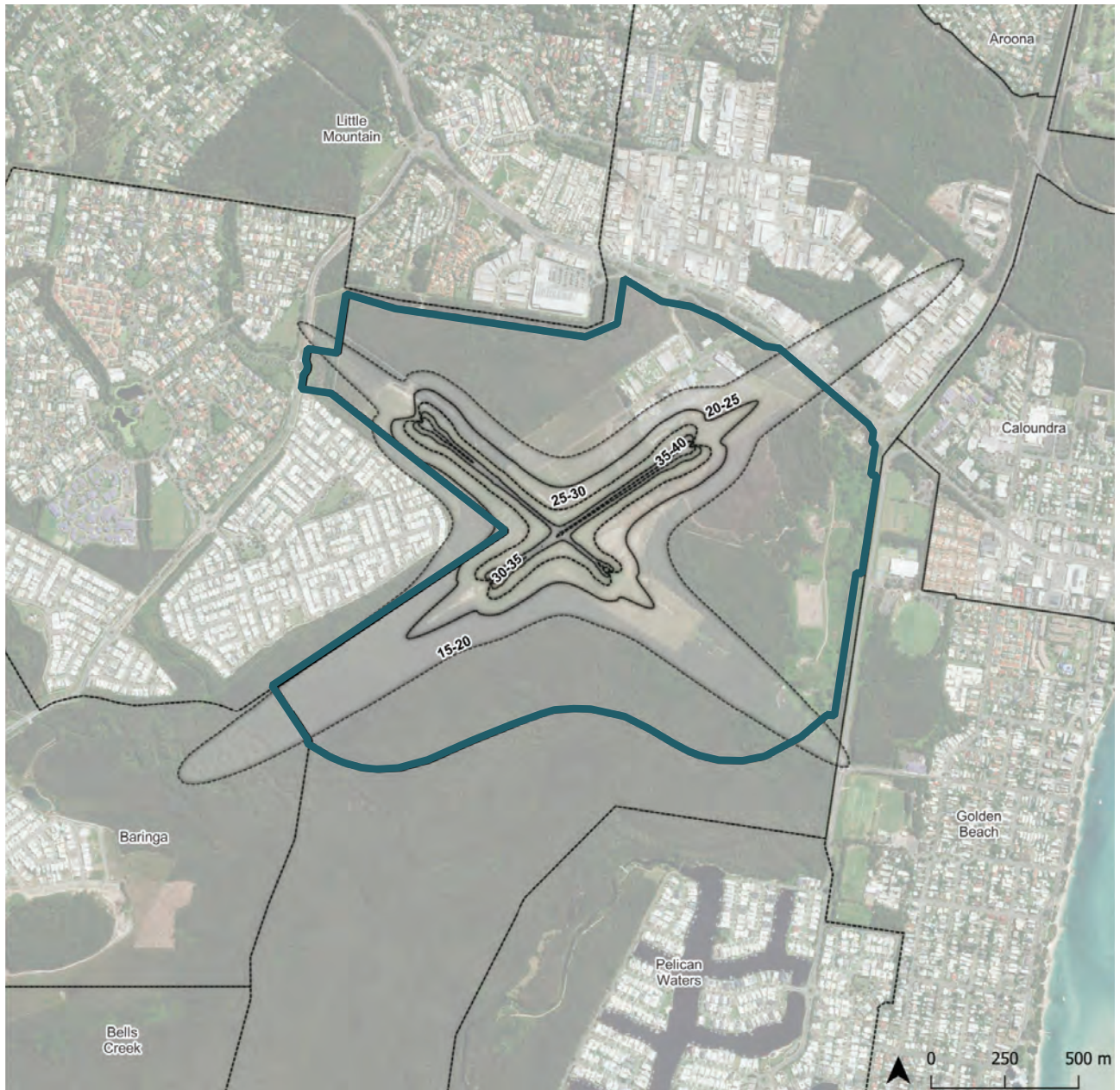
Figure 19: Caloundra Aerodrome Australian Noise Exposure Forecast Contours – Existing ( Sunshine Coast Planning Scheme 2014 extract )
