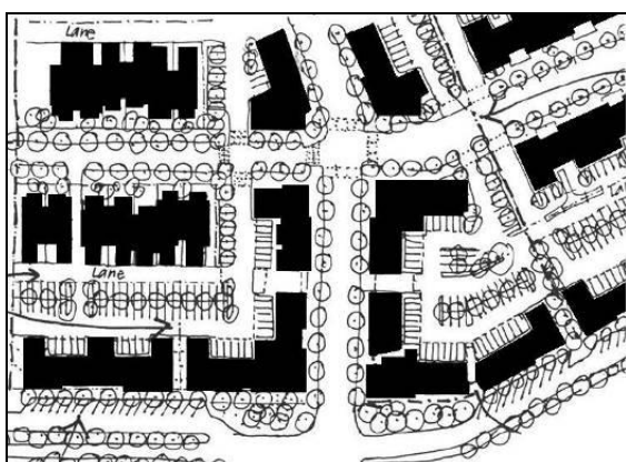
Figure SC6.3I Perimeter block form
