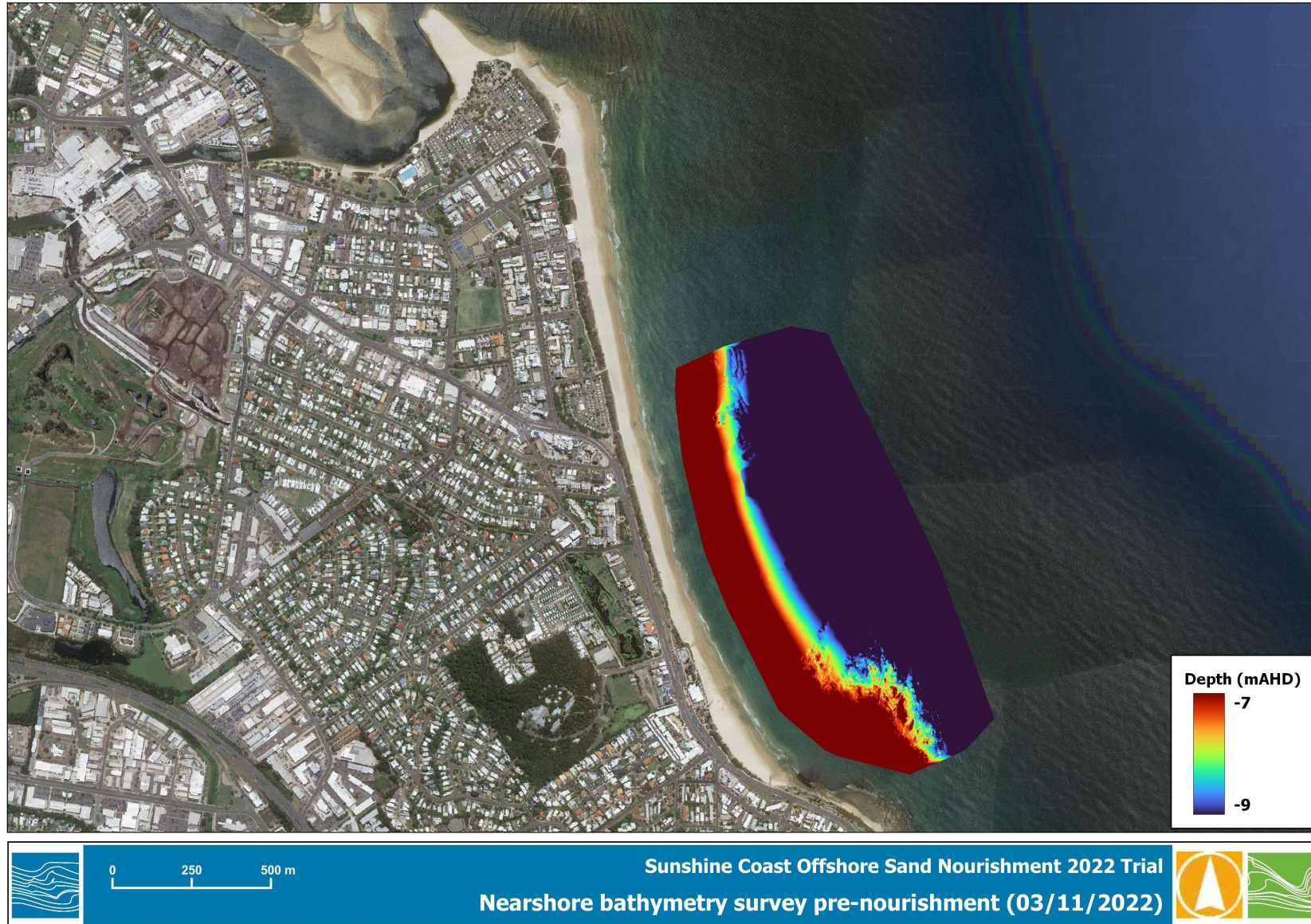
Figure 4-2 Pre-nourishment Multi-Beam Echo Sonar survey
