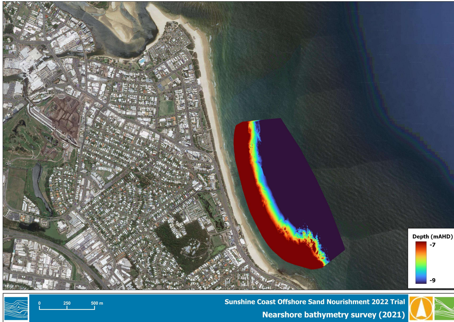
Figure 4-1 Multi-Beam Echo Sonar Survey, 2021
