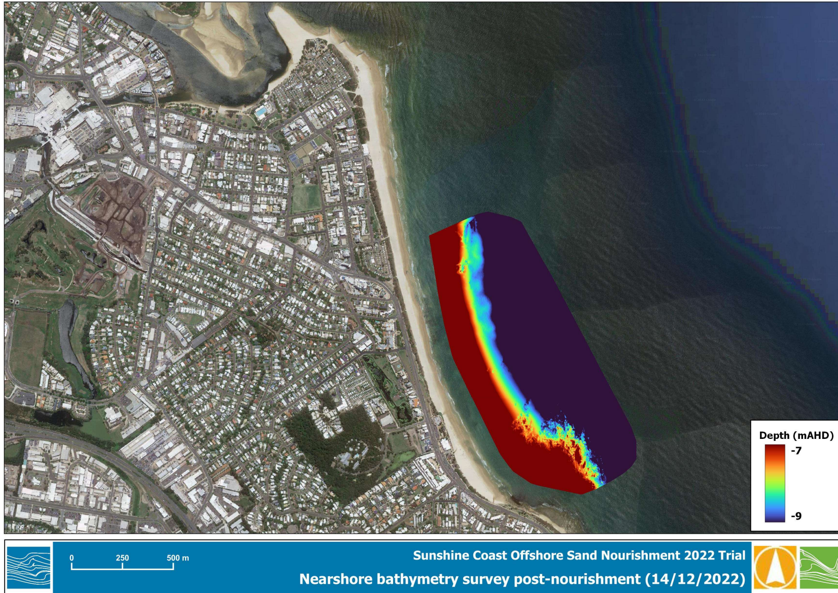
Figure 4-4 Post-nourishment Multi-Beam Echo Sonar survey - 24 days
