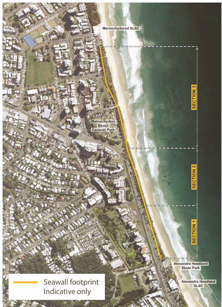
Figure 2: sections of the future buried seawall
