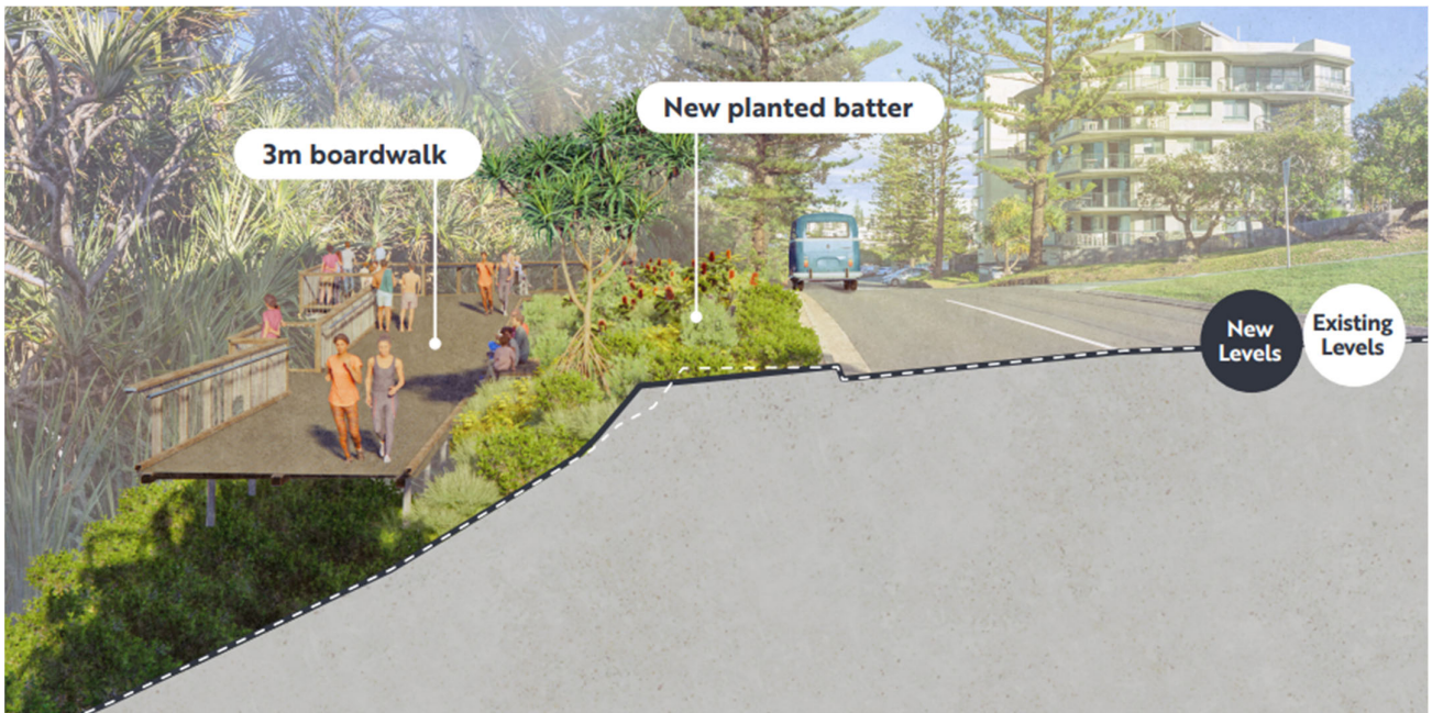
Figure 3 Artist's impression showing pathway transitioning to boardwalk adjacent to the existing road (Esplanade)
